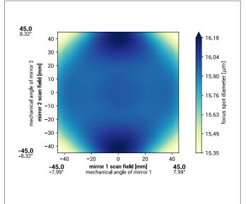
spot diameter at 86.5% level for a Gaussian beam ( $M^2 = 1$ ) with 10.0 mm diameter at  $1/e^2$ , clipped at 10.0 mm field size and mirror distances as given above for a two mirror scan system
